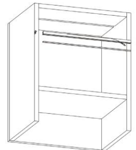
Install LED Tape, End Caps, Cover
