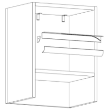
Step 1: Secure the mounting clip Step 2: Install the LED strip, plug, PC cover, fix the light body Step 3: Connect the driver and turn on the power supply
