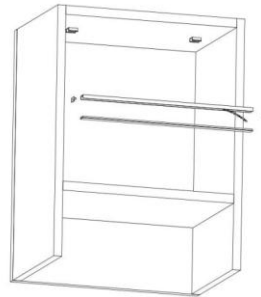
Step 2: Install the LED strip, plug, lampshade, fix the light body
